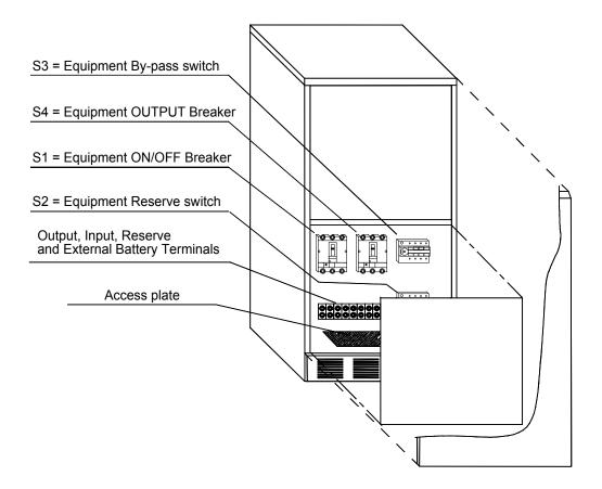
Figure 22 - 36 - 24/30/36kVA: Connections
